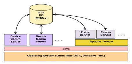
This graphic describes the basic system architecture of the **OpenGTS** system. The various device communication servers (the modules which listen for incoming data from the remote GPS tracking devices) run as separate processes on top of Java. The Track servlet (ie. The web-interface), as well as other servlets (including any http-based device communication server), run within a Servlet Container, such as Apache Tomcat.
